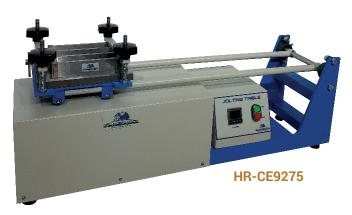
Jolting Table Apparatus with Soundproof Safety Cabinet is also available. The cabinet is lined internally with soundproofing material to reduce sound level conforming to CE directives.
