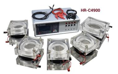
Rapid Chloride Permeability Tester has 4 pcs. sturdy, transparent cells, temperature sensor for each cell pair, sample connecting Apparatus, Sealing gaskets, voltage supply inputs and different colors inputs for polarities.
